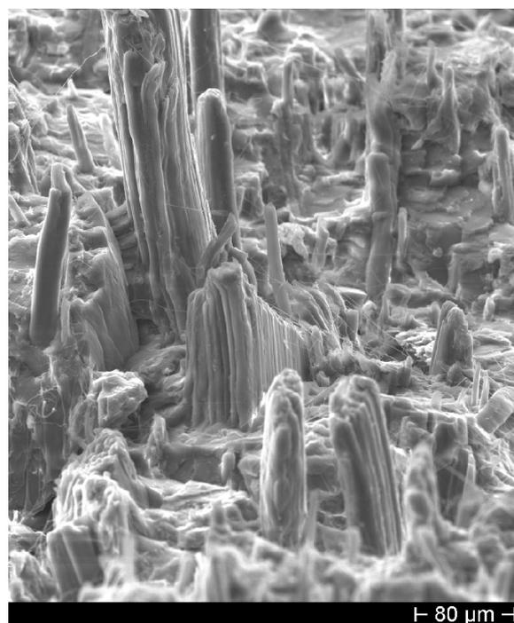
**Figure 1.** Fracture surface of poly(lactic acid)/phormium (30wt%) showing extensive fiber pull-out.
