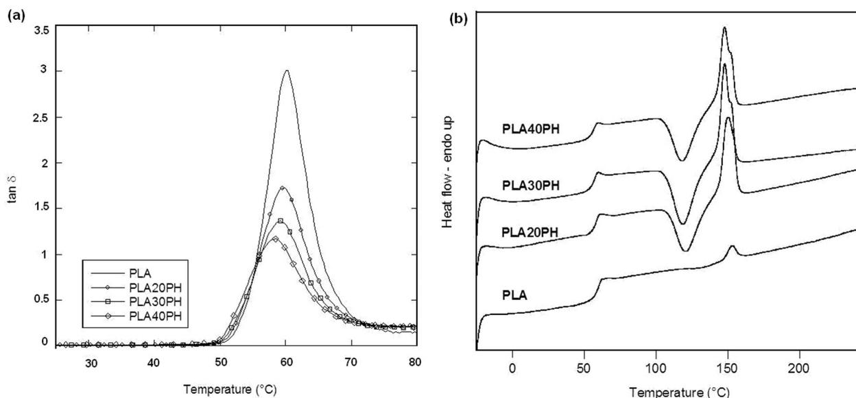
**Figure 2.** (a)  $\tan \delta$  vs. temperature curve (dynamic mechanical analysis), and (b) differential scanning calorimetry curves for all composites. PLA: Poly(lactic acid). PH: Phormium content.
