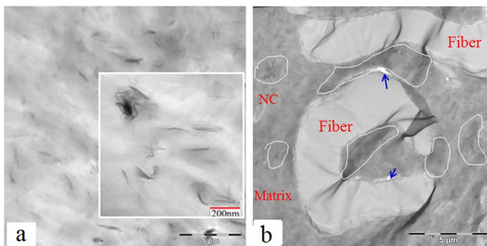
**Figure 2.** Tunneling electron microscope (TEM) images of the distribution of components in a polyethylene (PE) hybrid. (a) PE filled with nanoclay (NC) without additives and natural fibers, and (b) PE filled with additives and natural fibers in addition to NC.
