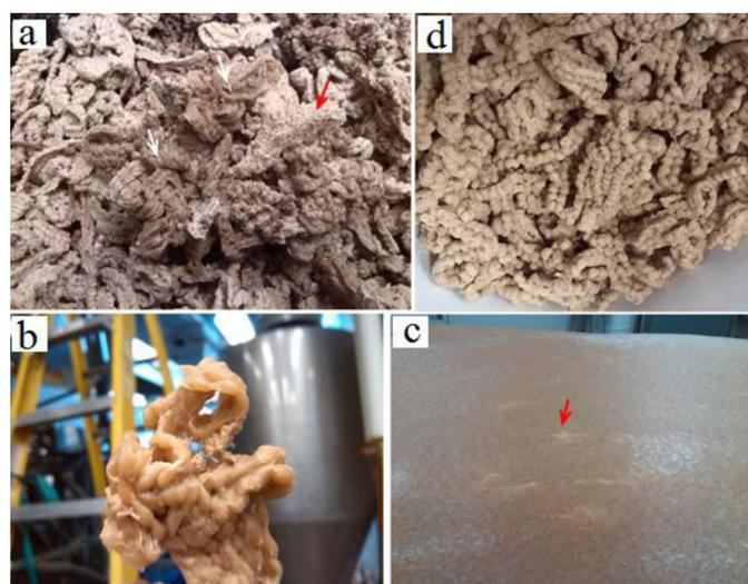
**Figure 1.** Typical extrusion compounding and processing of wood-plastic composite (WPC). Improper extrusion compounding is shown in (a). The red arrow points to fiber aggregation, and the white arrows indicate segments with too high a concentration of polymer. (b) Detail of segments with too much polymer; (c) a non-uniform extruded sheet using improperly compounded pellets, and (d) normal composite material.
