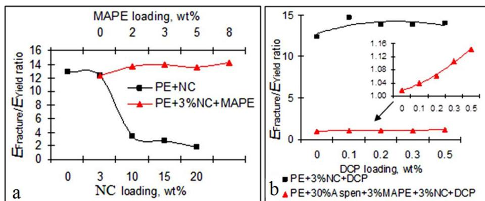
**Figure 3.** The plasticity of a PE hybrid upon the addition of maleated polyolefins (MAPE) and dicumyl peroxide (DCP), as expressed as the ratio of fracture energy to yield energy. (a) MAPE in PE nanocomposites, (b) DCP in a PE hybrid.
