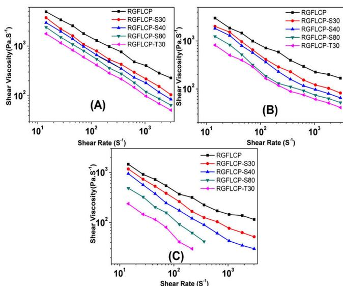
**Figure 5.** Rheological behavior of RGFLCP and its extruded samples: (A) 320°C, (B) 330°C, and (C) 340°C.
