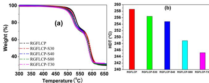
**Figure 4.** Thermal properties of RGFLCP and its extruded samples. (a) Thermogravimetric curves. (b) Heat deflection temperature (HDT).
