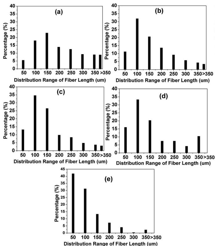
**Figure 2.** The glass fiber length distribution of recycled glass-fiber-reinforced liquid crystal polymer (RGFLCP) and extruded samples, where the final characters indicate the screw used during the extrusion. (a) RGFLCP, (b) RGFLCP-S30, (c) RGFLCP-S40, (d) RGFLCP-S80, and (e) RGFLCP-T30.
