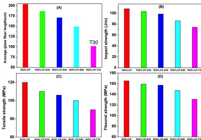
**Figure 3.** (A) Average glass fiber length ( $\bar{L}$ ), (B) impact strength, (C) tensile strength, and (D) flexural strength of RGFLCP and its extruded products. Red: RGFLCP. Green: RGFLCP-S30. Blue: RGFLCP-S40. Cyan: RGFLCP-S80. Pink: RGFLCP-T30.
