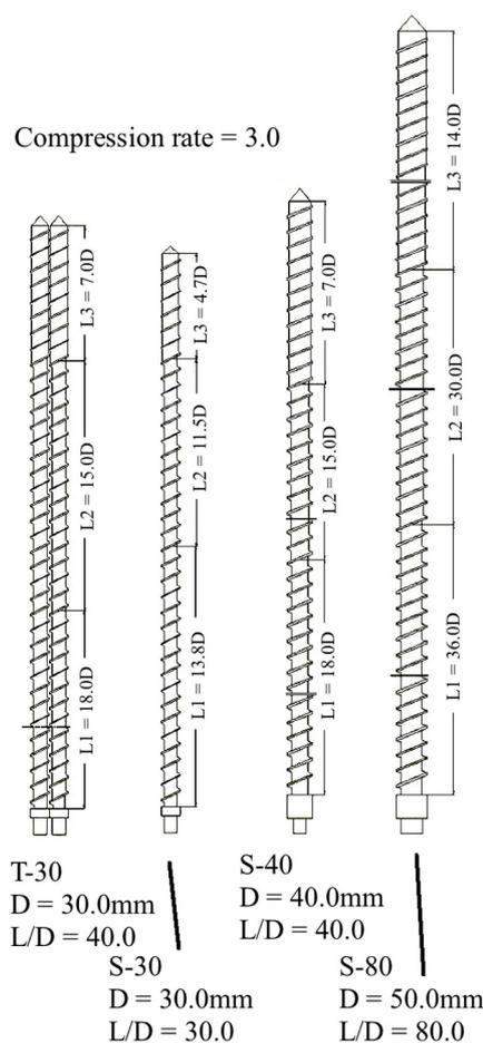
**Figure 1.** The structures of the different screws used in this investigation.  $L_{1,2,3}$ : Lengths of sections of the screws.  $D$ : Diameter.  $L/D$ : Length-to-diameter ratio. T-30, S-30, S-40, S-80: Abbreviated names for the different screws, where S means single and T means twin, and the two-digit number gives the ratio of the total length to the diameter.
