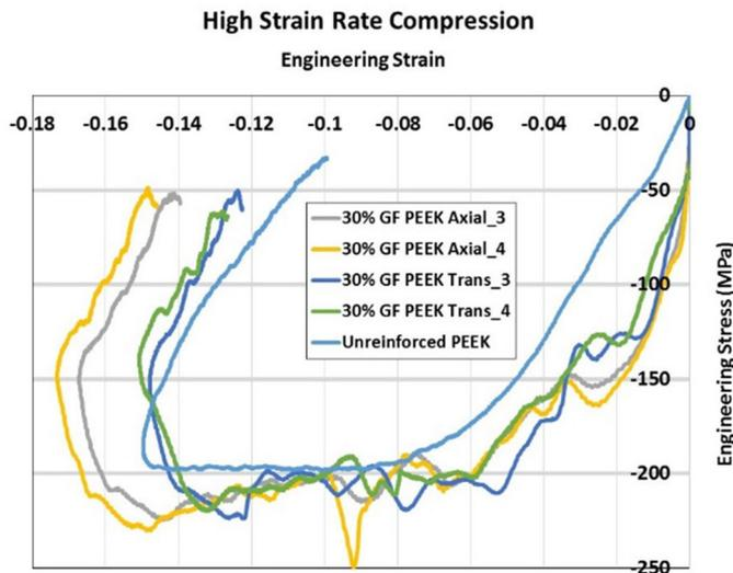
**Figure 2.** Compressive stress/strain at an approximate strain rate of 800 inverse seconds for the 30% glass-fiber-reinforced PEEK and unreinforced PEEK samples.
