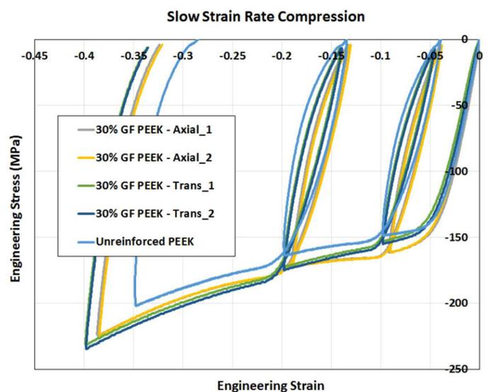
**Figure 1.** Compressive stress/strain at a strain rate of 0.01 inverse seconds for 30% glass-fiber-reinforced polyetherether ketone (PEEK) and unreinforced PEEK samples. The reinforced samples were tested in both the transverse (trans) and axial directions. GF: Glass fiber.
