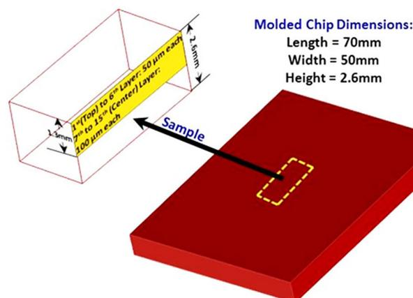
**Figure 1.** Schematic of molded plaque and location of thin sections.
