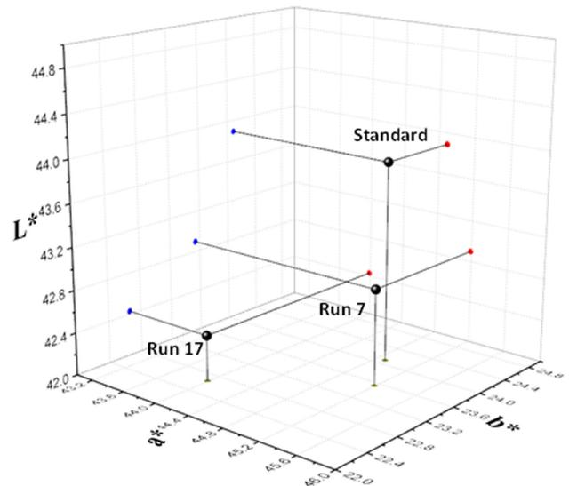
**Figure 5.** Sample color data and the standard reference in International Commission Illumination (CIE) L\*a\*b\* color space, where L\* is the illumination axis, and a\* and b\* the green/red and blue/yellow axes, respectively.
