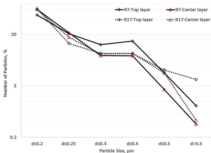
**Figure 3.** Plots of particle size (diameter, *d*) distribution for different layers and runs. R7, R17: Data from run 7 and run 17, respectively.
