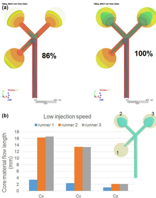
**Figure 2.** (a) Filling behavior and core penetration during injection molding at various total volume ratios. The yellow and orange represent the skin-layer material, which is injected first. The greens represent the subsequently injected core material. (b) Core penetration in three directions ( $C_x$ ,  $C_y$ , and  $C_z$ ) at injection speeds of  $10\text{cm}^3/\text{s}$ .
