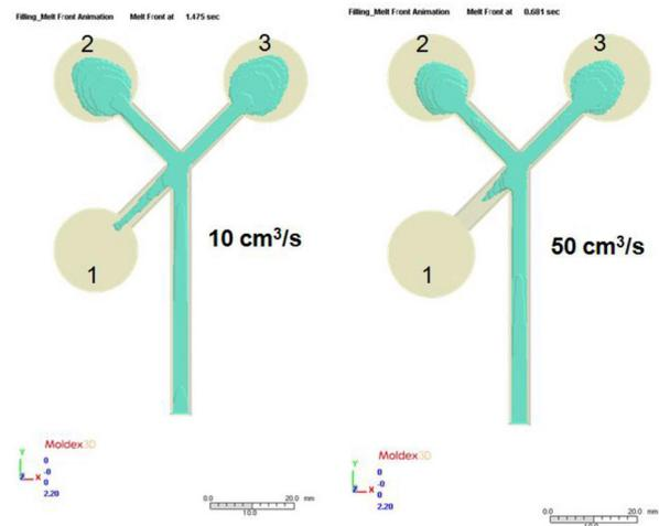
**Figure 3.** The effect of different injection speeds on core-penetration behavior. The first-shot material (skin layer, cream) is injected first, followed by the second-shot material (core material, green).
