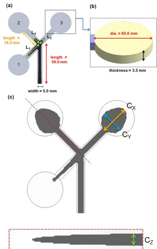
**Figure 1.** (a) Geometry of the co-injection multi-cavity system.  $L_1$ ,  $L_2$ , and  $L_3$ : Runners through which the material travels to get to the cavities 1, 2, and 3, respectively. (b) Cavity dimensions. (c) Core material penetration length at the end of filling.  $C_X$ ,  $C_Y$ , and  $C_Z$ : Core penetration lengths in the X, Y, and Z directions, respectively.
