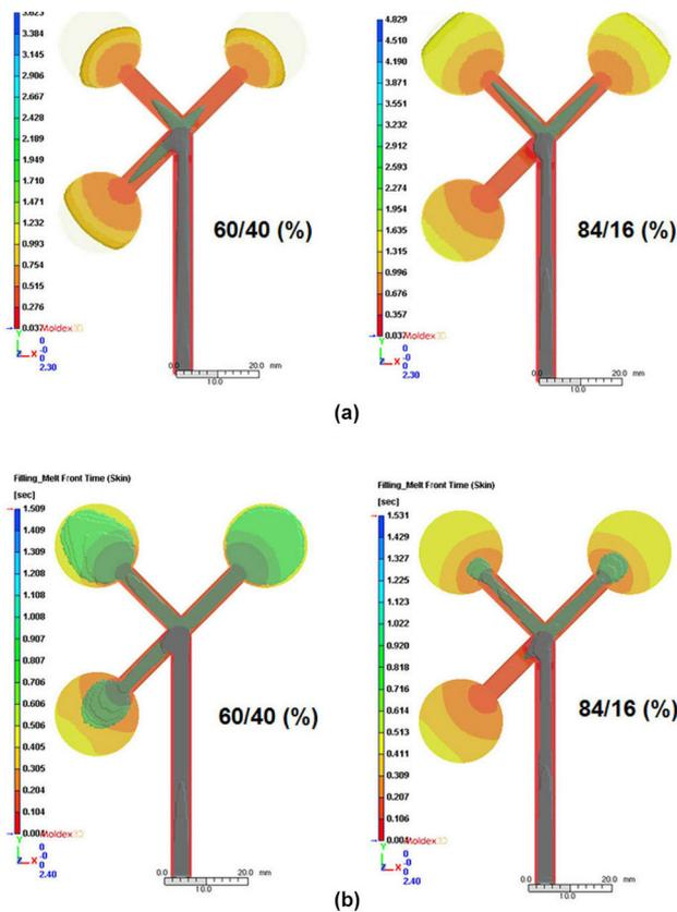
**Figure 4.** The simulated melt front under different skin/core material volume ratios. Core-material penetration length when (a) one of the branches first reaches a cavity and (b) at the end of filling.
