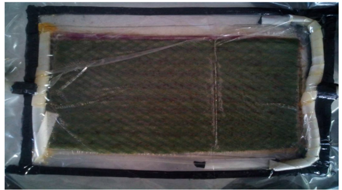
Figure 1. Photograph illustrating the vacuum infusion process setup. A vacuum bag covers the entire mold, including the sealant tape.
