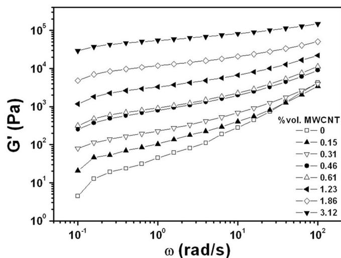
**Figure 1.** Storage modulus ( $G'$ ) measurements, as a function of angular frequency ( $\omega$ ), for polyamide 12/polyamide 6 (PA12/PA6) composites with varying multiwall carbon nanotube (MWCNT) contents, expressed as volume % (%vol). The measurements were obtained at 235°C, with a TA Instruments ARES rheometer (25mm parallel plate and 1mm gap).
