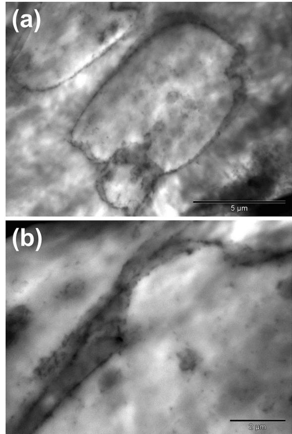
**Figure 3.** Transmission electron microscope images of (a) the PA12/PA6/MWCNT composite containing 0.46%vol CNT particles, and (b) a close-up image of the interface between the two polyamide phases. Images were obtained using a JEOL JEM-1010 instrument.
