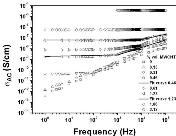
**Figure 2.** Experimental results illustrating the frequency dependence of conductivity ( $\sigma_{AC}$ ) for the PA12/PA6 composites with different MWCNT contents. Measurements were made on a TA Instruments dielectric analyzer (DEA 2970 iv). AC: Alternating current.
