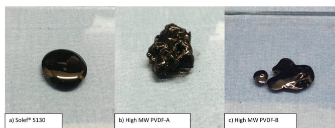
Figure 1. Photographs of the slurries (about 20mm in diameter) prepared with different polyvinylidene difluoride (PVDF) binders. (a) Slurry produced by emulsion polymerization with Solvay Solef 5130 (molecular weight, MW, >900,000). (b) PVDF-A slurry (MW>900,000) produced by emulsion polymerization. (c) PVDF-B slurry (MW>1,000,000) produced by suspension polymerization.
