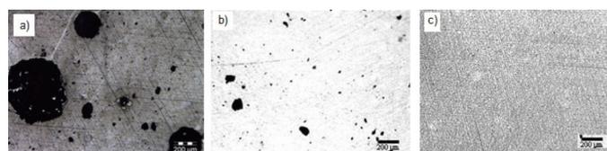
**Figure 1.** Example optical microscope images of the multiwall carbon nanotube/polypropylene (MWCNT/PP) nanocomposite samples. These samples were produced under (a) high-shear, (b) mid-shear, and (c) low-shear conditions. Scale bars indicate 200 μm.
