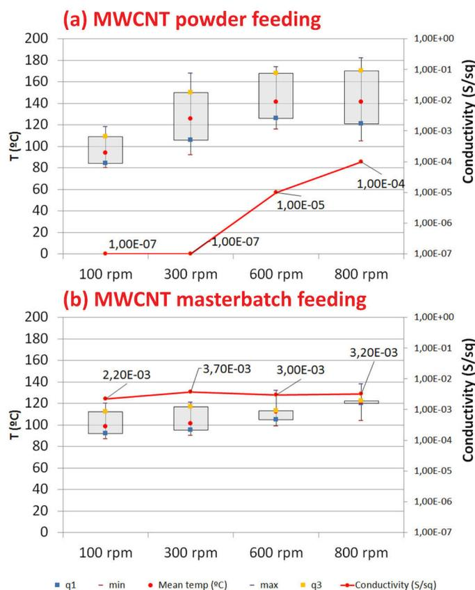
**Figure 3.** Temperature ( $T$ ) and conductivity of the nanocomposites at different screw-speed extrusion conditions (after 60s of microwave heating). Samples were obtained by (a) direct feeding of MWCNT powder and (b) MWCNT masterbatch feeding.  $q1$  and  $q3$ : First and third quartiles (i.e., 25 and 75% of the sample, respectively).
