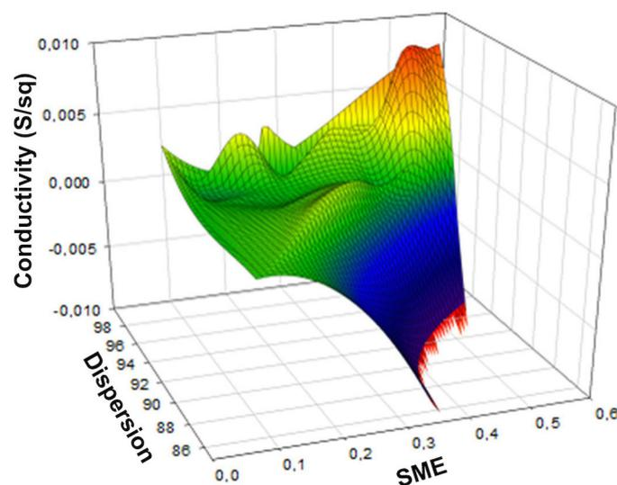
**Figure 2.** Correlation between the specific mechanical energy (SME), dispersion factor, and surface electrical conductivity MWCNT/PP nanocomposites. S/Sq: Siemens/square.
