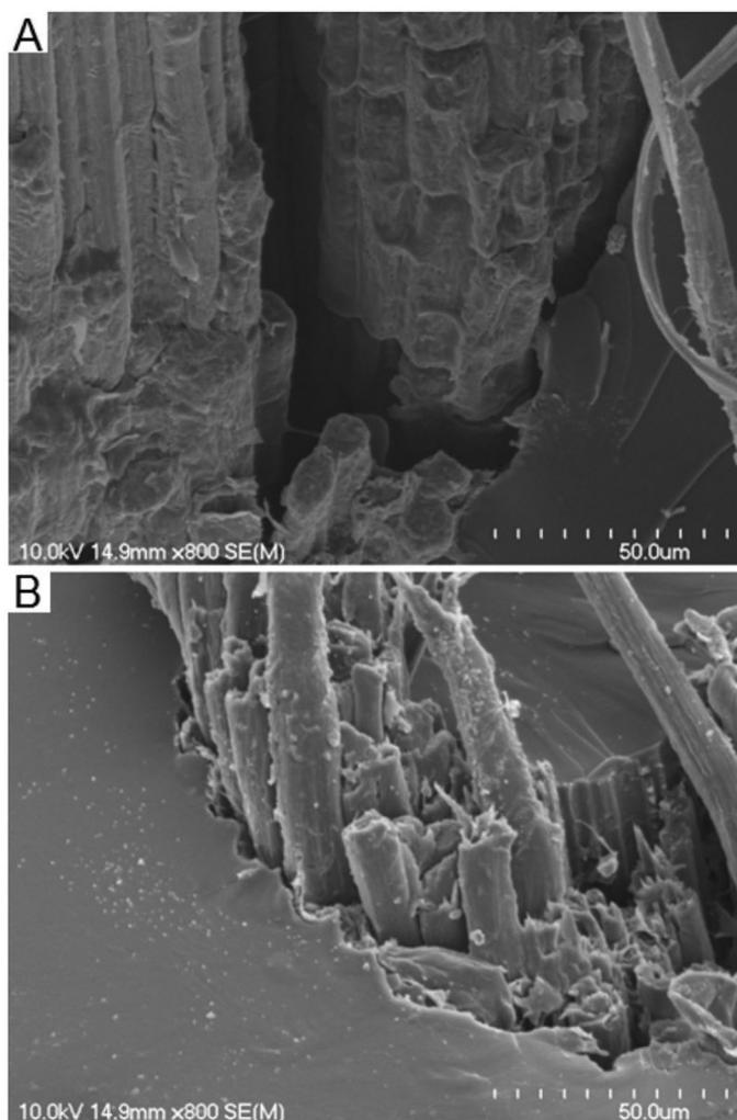
**Figure 3.** Scanning electron microscope images of the failure area (after flexion) in BF composites made with (a) epoxy-coated fibers and (b) nanoreinforced fibers.
