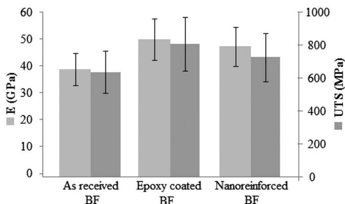
**Figure 2.** Young's modulus ( $E$ , light gray) and ultimate tensile strength (UTS, dark gray) of uncoated (i.e., as received), epoxy-coated, and nanoreinforced (i.e., coated with an epoxy/ $\text{SiO}_2$  composite) BF bundles.
