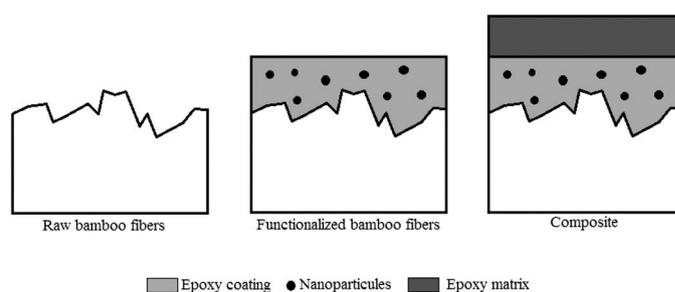
**Figure 1.** Schematic illustration of the bamboo fiber (BF) coating process. First, the raw BFs are coated with an epoxy/silicon dioxide ( $\text{SiO}_2$ ) nanoparticle suspension. The coated fibers are then immersed in the epoxy, which makes up the matrix of the composite. After a few hours, the composite is fully cured and ready to be tested.
