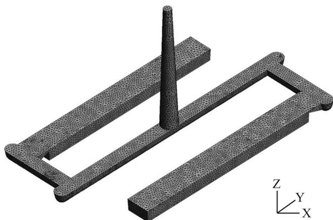
**Figure 2.** Computer-aided design model and finite element method mesh used for the simulations of the rectangular impact bars.
