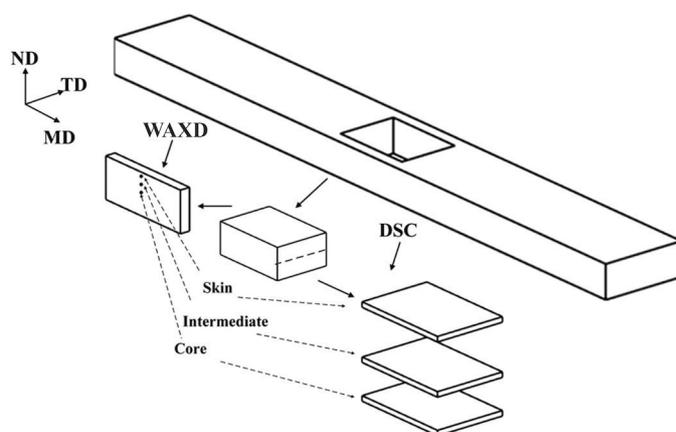
**Figure 1.** Schematic diagram illustrating the different sections within the  $\beta$ -nucleated isotactic polypropylene (iPP) injection-molded samples, at which wide-angle x-ray diffraction (WAXD) and differential scanning calorimetry (DSC) measurements were obtained to quantify the crystallization. MD: Molding direction. TD: Transverse direction. ND: Normal direction to the MD–TD plane.
