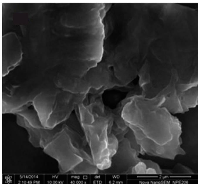
**Figure 1.** Scanning electron microscope image of graphene oxide (GO) particles used in the polytriazoleimide (PTAI) nanocomposites.<sup>5</sup>
