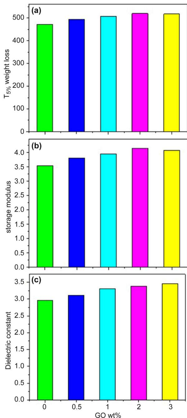
**Figure 2.** Illustrating the (a) thermal properties, (b) results of a dynamic analysis, and (c) dielectric constants of the PTAI/GO nanocomposites. T<sub>5%</sub>: Temperature at which 5% mass loss occurs. wt%: Weight percent (i.e., concentration).<sup>5</sup>
