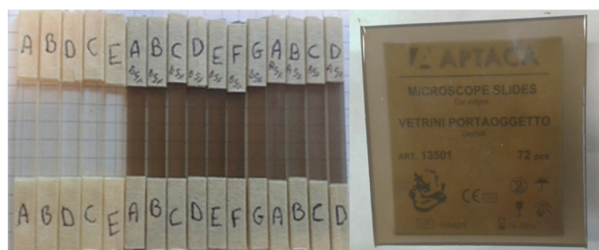
Figure 1. Left: Several examples of samples used in the study. The pure epoxy resin samples are shown on the far left (labeled A–E). The nanocomposite samples containing 3wt% bentonite-6-(4-butylphenyl)-1,3,5-triazine-2,4-diamine (R-BeBFTDA) and bentonite-11-amino-N-(pyridine-2yl)undecanamide (R-BeAPUA) are shown in the center (A–G) and on the right (A–D), respectively. Right: Photograph illustrating the transparency of the 3wt% R-BeAPUA panel used in the fire behavior tests.
