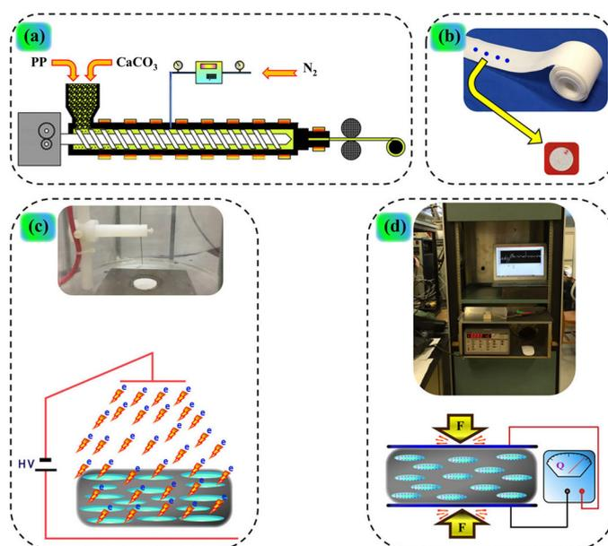
**Figure 1.** (a) Schematic representation of the developed foam extrusion process to obtain thin polypropylene (PP) films with an eye-like cellular structure, (b) foamed PP film and sample for charging, (c) corona charging system, and (d) piezoelectric measurement system. CaCO<sub>3</sub>: Calcium carbonate (nucleating agent). N<sub>2</sub>: Nitrogen. HV: High voltage. e: Electron. F: Force. Q: Electrical charge.
