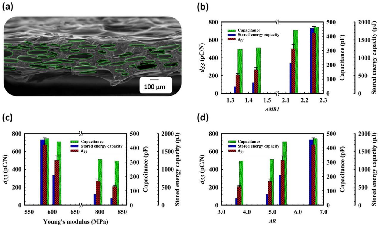
**Figure 2.** (a) Typical scanning electron microscope image in the machine direction of a PP film having a well-developed eye-like cellular structure, and the piezoelectric  $d_{33}$  coefficient, capacitance, and stored energy capacity of the cellular PP films as a function of (b) AMRI, (c) Young's modulus, and (d) AR value. AMR: Anisotropic modulus ratio. AR: Aspect ratio.
