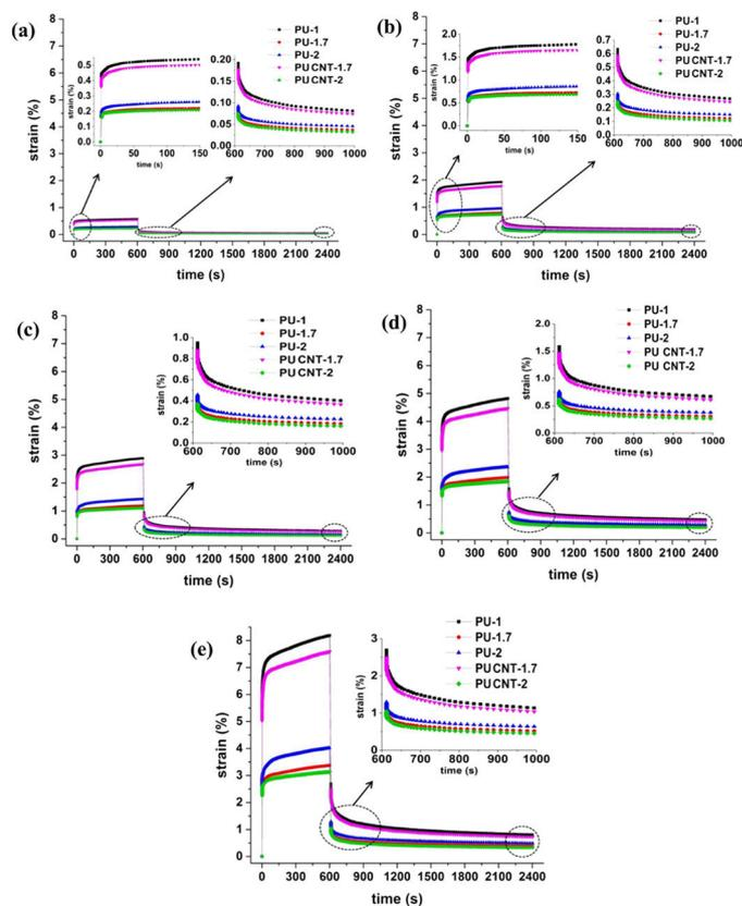
**Figure 1.** Experimentally measured creep and creep-recovery strain, as a function of time, for the polyurethane (PU) and PU/multiwalled carbon nanotube (CNT) nanocomposites at 30°C. Results are shown for stress levels of (a) 0.5MPa, (b) 1MPa, (c) 1.5MPa, (d) 2MPa, and (e) 2.5MPa. Sample details are given in Table 1.
