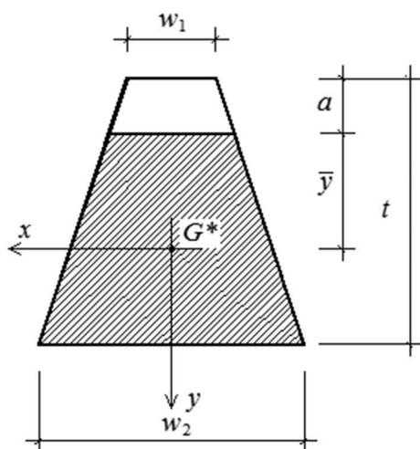
**Figure 2.** Cross section (in the  $x$ - $y$  plane) of a cracked trapezoidal silicon nanobeam, showing the parameters used in the theoretical model for predicting the bending strength of a cracked nanobeam.  $G^*$ : Center of mass.  $a$ : Crack length.  $\bar{y}$ : Crack tip coordinate,  $y$ : Height of trapezoid.  $w_1$ ,  $w_2$ : Width of the top and bottom of the trapezoid, respectively.
