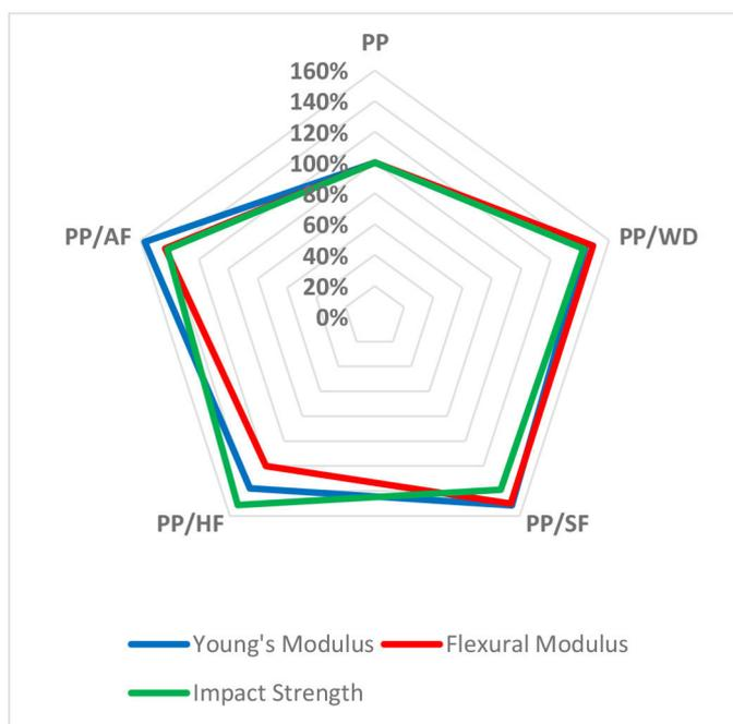
**Figure 2.** Mechanical characteristics of polypropylene (PP) were significantly improved when it was combined with either wood dust (WD) or wheat straw fibers. PP/X: Compound of 80wt.% PP and 20wt.% X.
