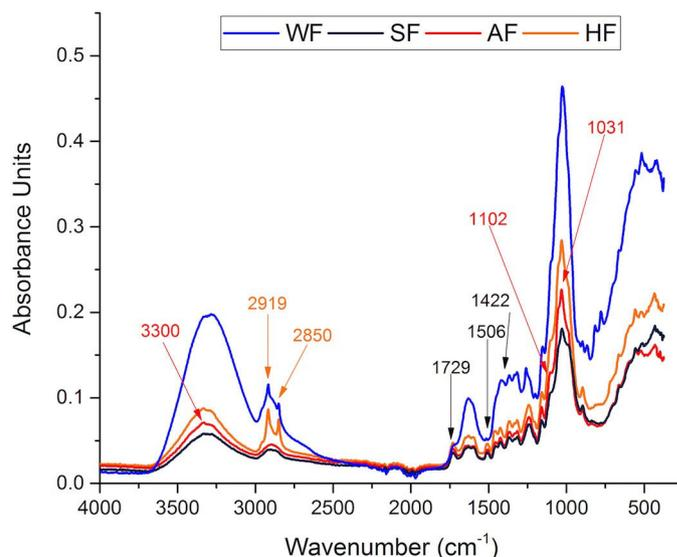
**Figure 1.** Spectra obtained by attenuated total reflectance infrared spectroscopy (ATR-IR) of four types of wheat straw fiber (see Table 1 for key). The spectra confirm the chemical characteristics of the modified wheat straw fibers
