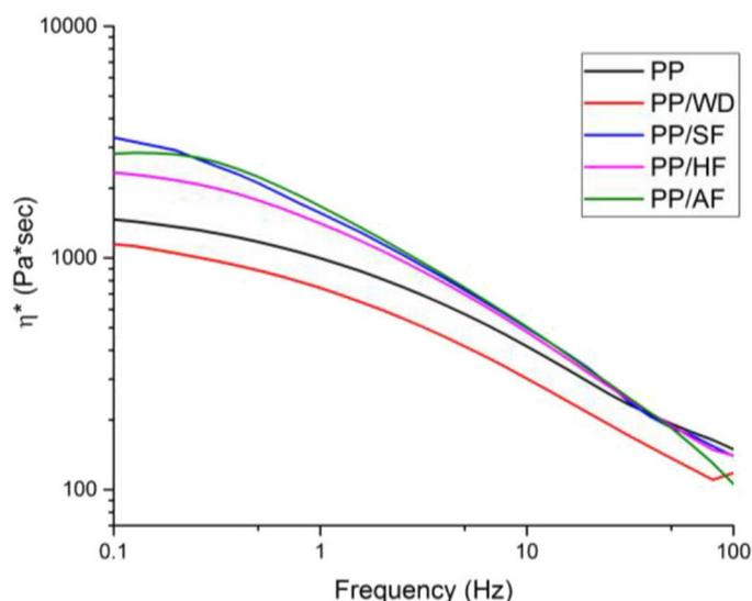
**Figure 3.** Complex viscosity ( $\eta^*$ ) of the materials at 220°C measured by parallel-plate rheometry. Adding wheat straw fibers to PP increased the complex viscosity at lower shear rates (lower frequencies). By contrast, adding wood dust decreased the viscosity.
