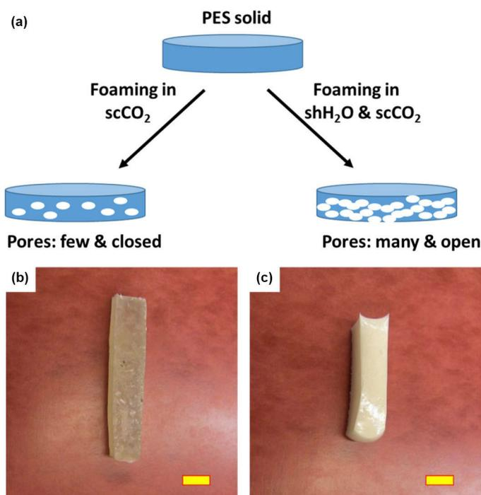
**Figure 1.** (a) Illustration showing the results obtained in polyethersulfone (PES) foamed with supercritical carbon dioxide (scCO<sub>2</sub>), and with comedia of scCO<sub>2</sub>/superheated water (shH<sub>2</sub>O). Photographs show PES in the form of (b) a solid block (after treatment with scCO<sub>2</sub>) and (c) foam (after treatment with scCO<sub>2</sub>/shH<sub>2</sub>O comedia).
