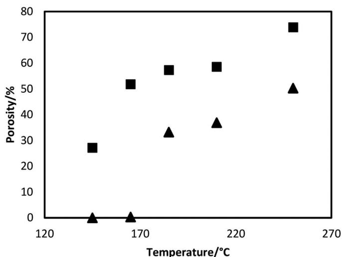
**Figure 2.** Porosity vs. foaming temperature in PES processed with  $scCO_2$  (triangles) and  $scCO_2/shH_2O$  (squares).
