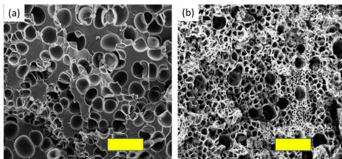
**Figure 3.** Scanning electron micrographs of cross sections of PES foamed with (a)  $scCO_2$  and (b)  $scCO_2/shH_2O$ . Scales are 50  $\mu m$ .
