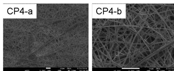
**Figure 3.** SEM images of NCTS/PVA after contact with platelet-rich plasma at different magnifications: (a) 650× and (b) 2500×.
