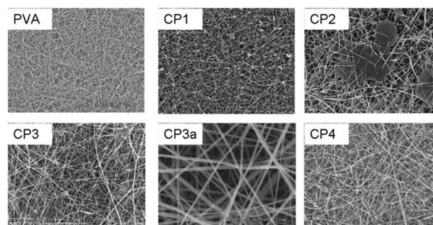
**Figure 1.** Scanning electron microscope (SEM) images of chitosan nanopowders/poly(vinyl alcohol) (NCTS/PVA) samples—with 8wt% PVA—prepared under different conditions (i.e., by varying the voltage and the distance between the injector and collector, respectively, during electrospinning) at a magnification of 1500 $\times$ . PVA: 30kV, 22cm. CP1: 30kV, 10cm. CP2: 35kV, 10cm. CP3: 35kV, 16cm. CP3a: Magnification of CP3 (10,000 $\times$ ). CP4: 40kV, 16cm.
