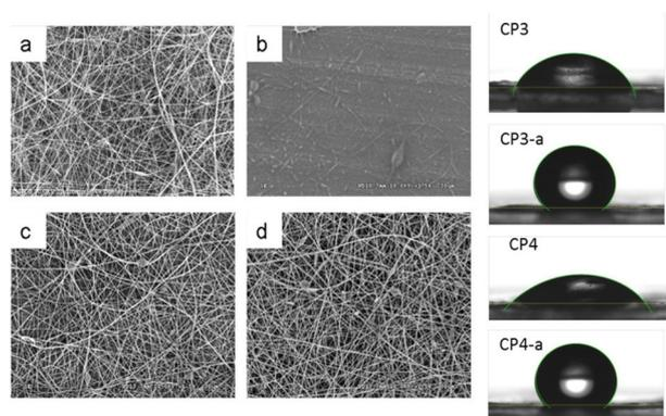
**Figure 2.** SEM images of samples before and after they were processed with water. CP3 (a) before and (b) after processing with water. Crosslinked CP3 (CP3-a) (c) before and (d) after processing with water. The water contact angles of the mats are also shown (right panel). CP4-a: Crosslinked CP4.
