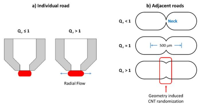
**Figure 1.** Schematic diagrams of hypothesized factors leading to carbon nanotube (CNT) misalignment during 3D printing: (a) radial flow occurring as the material overfills the gap, and (b) geometry-based fusion between adjacent roads.  $Q_r$ : Dimensionless volumetric flow rate.
