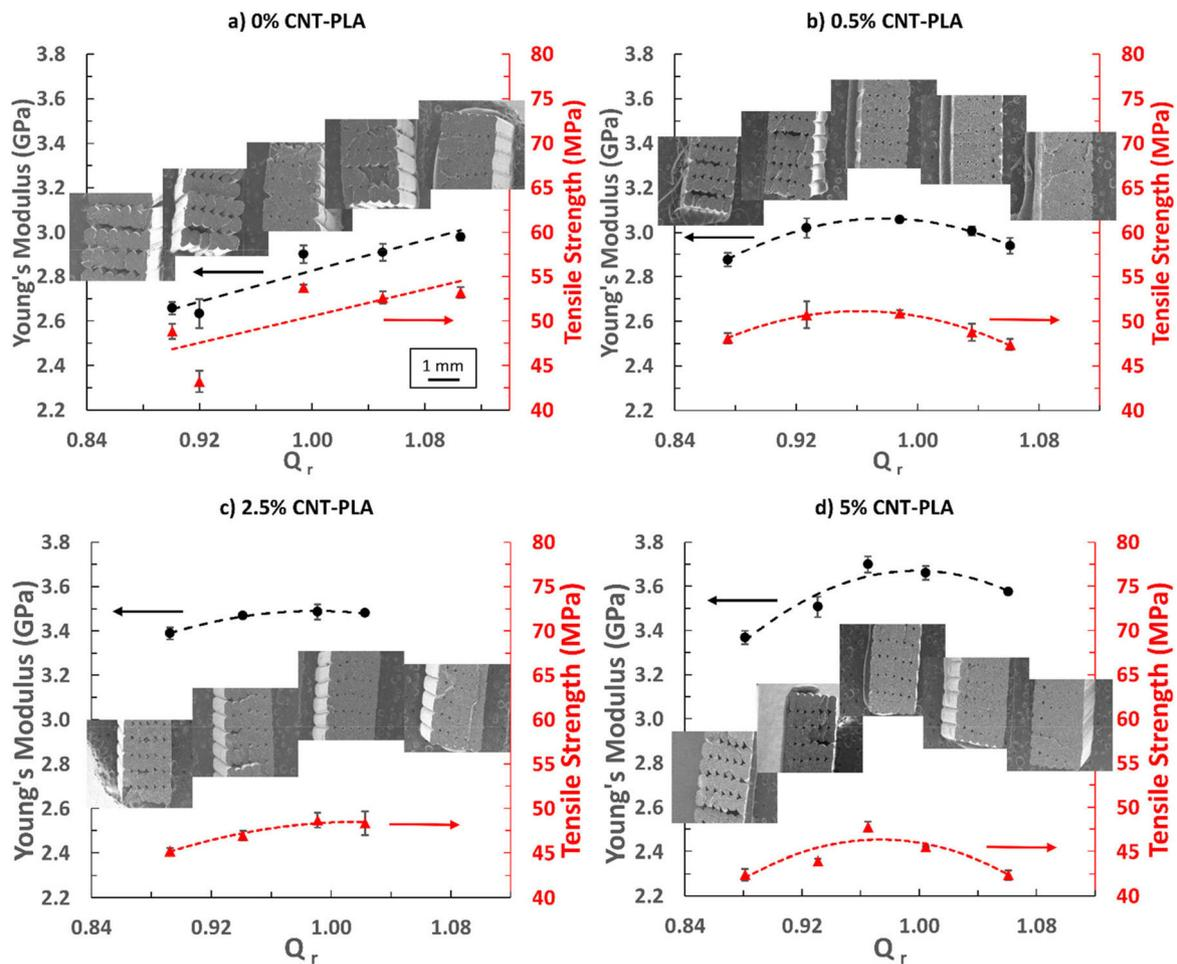
**Figure 2.** Young's modulus (black), tensile strength (red), and scanning electron microscope (SEM) images of the fractured surface as a function of dimensionless volumetric flow rate ( $Q_r$ ) for CNT/poly(lactic acid) (CNT-PLA) composites with varying CNT content (0–5%). (a) 0% CNT-PLA, (b) 0.5% CNT-PLA, (c) 2.5% CNT-PLA, and (d) 5% CNT-PLA, respectively. The scale shown in (a) applies to all SEM images.
