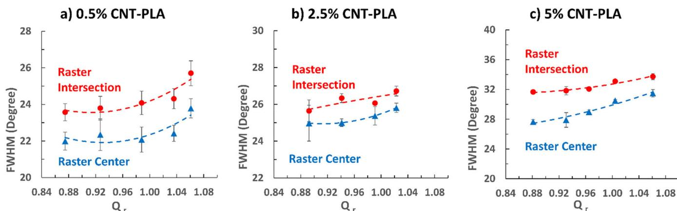
**Figure 3.** Full width at half-maximum (FWHM) of: (a) 0.5% CNT-PLA, (b) 2.5% CNT-PLA, and (c) 5% CNT-PLA as a function of  $Q_r$ . The error bar represents the standard deviation of at least three samples.
