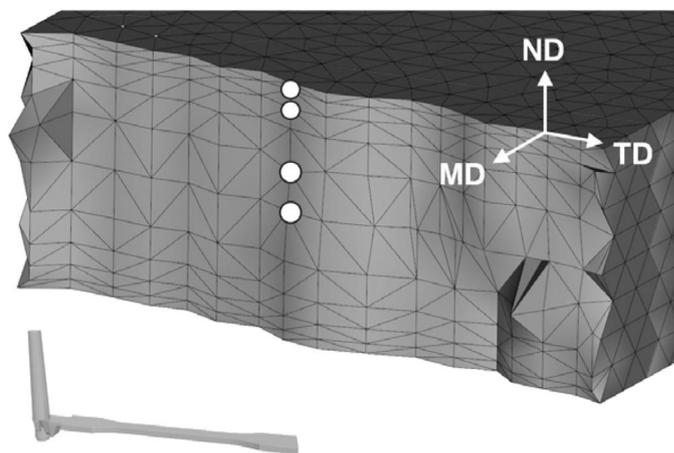
**Figure 1.** CAD 3D model (main image) of the molded polyamide 11 (PA11) specimen (inset bottom left) imported to Moldflow software and locations assigned for the simulation (white spots, top) at distances of 50, 200, 700, and  $1000\mu\text{m}$  from the surface. MD, ND, TD: Melt flow direction, normal to melt flow direction, and transverse to melt flow direction, respectively.
