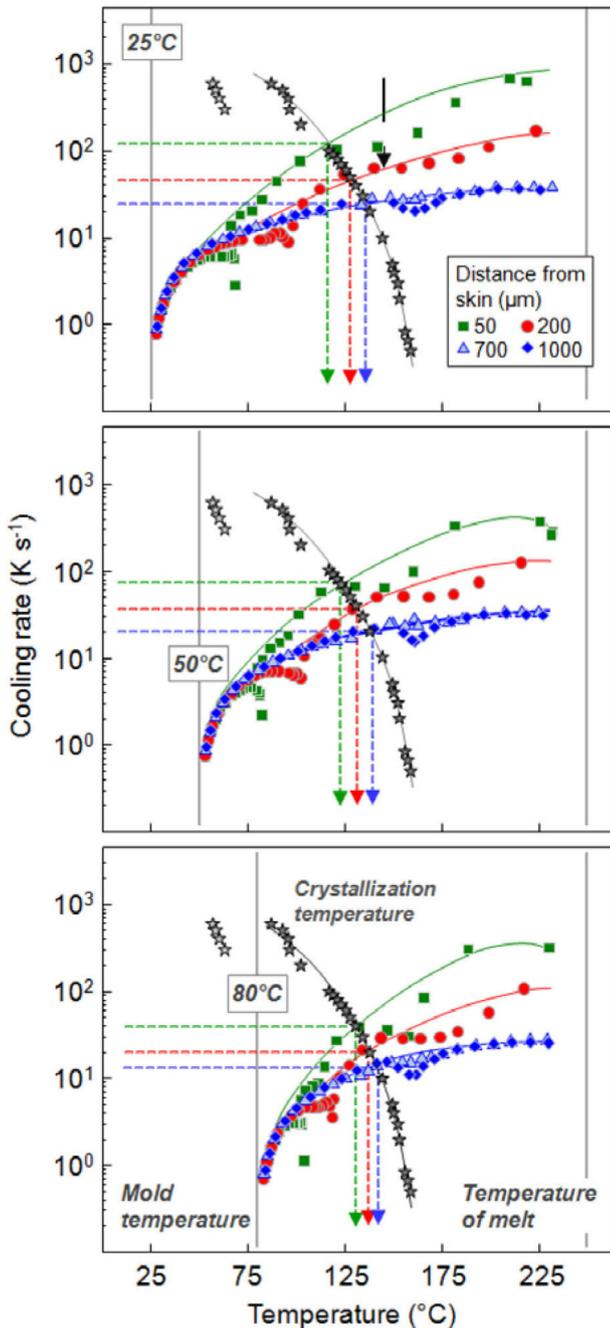
**Figure 2.** Simulated cooling rates during injection molding of PA11 at different distances from the mold wall shown by green (50 $\mu\text{m}$ ), red (200 $\mu\text{m}$ ), white (700 $\mu\text{m}$ ), and blue (1000 $\mu\text{m}$ ) symbols and lines for mold temperatures of 25 (top), 50 (middle), and 80 $^{\circ}\text{C}$  (bottom). The star symbols in each plot show temperatures of crystallization of PA11, which were measured as a function of cooling rate in a separate study.<sup>9</sup>
