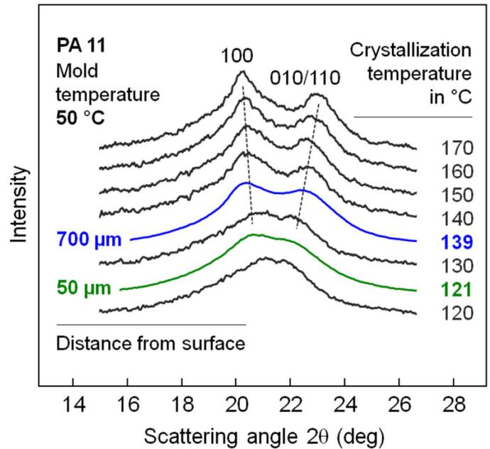
**Figure 3.** X-ray diffraction patterns of PA11 moldings prepared with a mold temperature of 50 $^{\circ}\text{C}$  taken at different distances from the surface of the 50 $\mu\text{m}$  (green) and 700 $\mu\text{m}$  (blue) fit well into a series of patterns for isothermally prepared PA11 of the same grade sorted by crystallization temperature.
